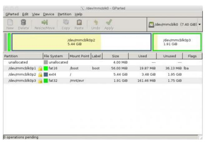
Select the correct device by selecting the 2nd option at the top right (under /dev/mmcblk0). Then you will see the new memory card. Resize the last partition on this card to the maximum size. Make sure to hit the "Apply" button afterwards. Then the card will be prepared (this can take a while).
