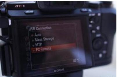
view". This will lead to an unwanted delay on your camera and your camera will not correctly take over the USB commands from the RamperPro:
