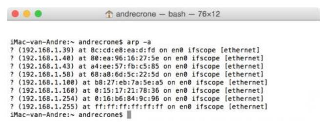
One of the IP addresses will be linked to your RamperPro. In this case its 192.168.1.100. Now you can startup the software that can prepare your memory card by entering this command in the terminal window: ssh -X ramperpro@192.168.1.100 gksudo gparted
