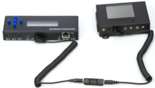
[69] The MX3 can also be connected to the RamperPro. This gives you a three axis motion control solution. Please note the direction of the O on the isolator.
