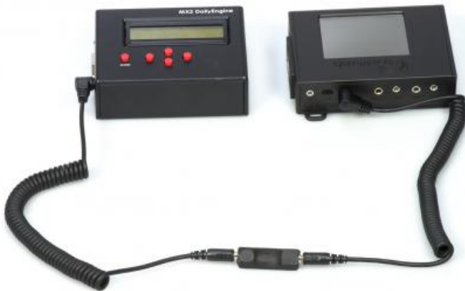
[68] The RamperPro connected to the MX2 motion controller. Please note the direction of the O on the I/O isolator.
