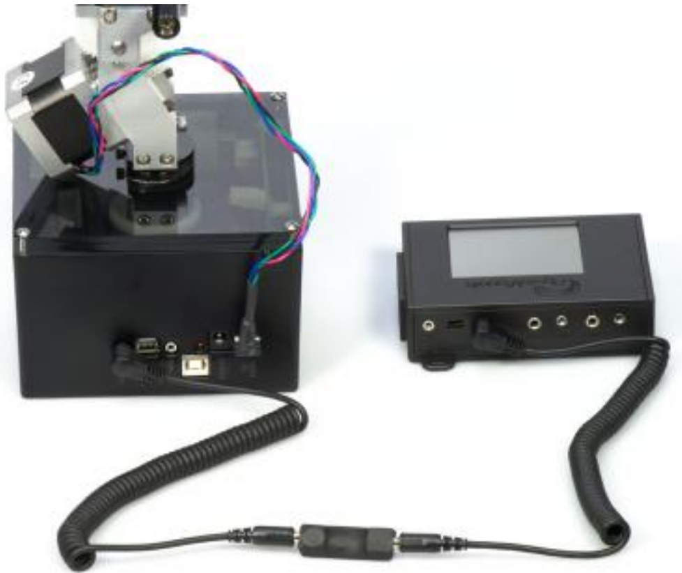
[70] The I/O isolator can also be used to interface the TB3. This way you get a three axis stepper motor solution. The RamperPro will trigger the TB3. This way the axis can move to the next position when the camera.
