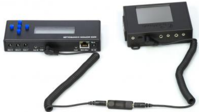
[69] The MX3 can also be connected to the RamperPro. This gives you a three axis motion control solution. Please note the direction of the O on the isolator.
