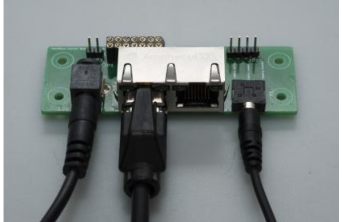
[8] A close-up of the ElysiaVisuals nanoMoco connector board. This board can be connected to the nanoMoco board. The power cable, nanoMoco USB-RS485 cable and the camera cable are connected here.
