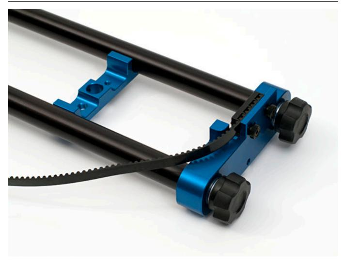
Feed the free end of the belt around the nearest idler and pull all of the slack belt through. Guide the loose end of the belt through the space between the idler and the pulley, and then around the pulley. Now, feed the belt fully around the pulley, and behind the second idler. With your free hand, push the cart away from the end of the slider where the belt is already clipped in to, to tension the belt on that side of the cart.
