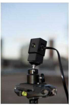
[1]This chapter gives you more details about the external light sensor. It also describes how to use the auto exposure mode of the RamperPro where the images from your camera are analyzed during a timelapse shoot. The combination of the light sensor and the auto mode are described by explaining what is happening during a sunset.
