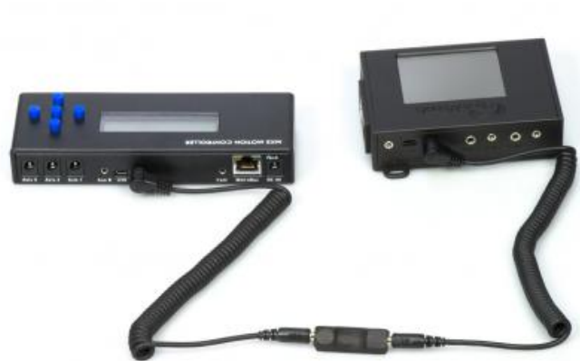
[10] The MX3 can also be connected to the RamperPro. This gives you a three axis motion control solution. Please note the direction of the O on the isolator.
