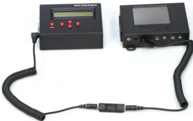
[9] The RamperPro connected to the MX2 motion controller. Please note the direction of the O on the I/O isolator.
