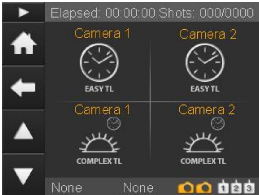
[5]The "CONFIG" button on the parameters screen leads to the screen on the left. The four icons will lead you to the parameters of the time lapse engines.
