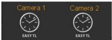
The basic intervalometer mode of the RamperPro gives you an intervalometer that can be used for "normal" timelapse sequences. Just set the interval between the images that you want to shoot and you are good to go. Don't forget to set the "Number of images" setting because that sets the amount of images that the basic intervalometer will take before it will automatically stop. Set this value to a high value if you don't know how many images you are going to take upfront.
