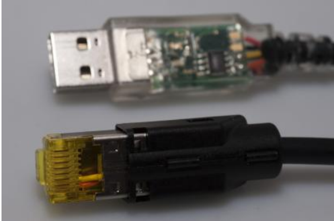
[7] Here you see a close-up of the nanoMoco USB-RS485 cable. This is a special cable that converts USB signals to RS485. A Hirose RJ45 plug is connected to the other side.
