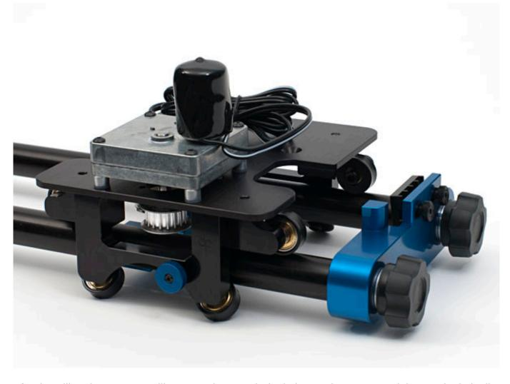
After installing the cart, you will now need to attach the belt. Starting at one end, loosen the belt clip and install one end of the belt into the clip such that the belt teeth and the clip teeth meet each other. Slide the belt clip so that it is closest to the belt guide, and then tighten the clip bolts tightly with your fingers. Guide the belt out and around the belt guide, and then to the cart.
