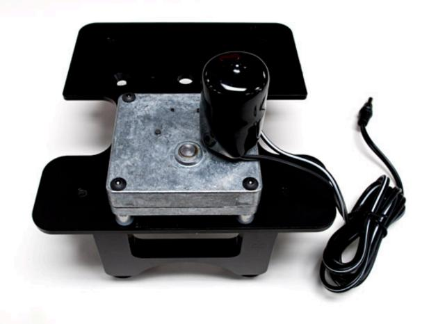
b. Using the provided hex tool, tighten down the bolts by starting at one corner, then moving to the opposite corner, until all four bolts have been started. Do not tighten down any bolts fully until the all four bolts have been started.
